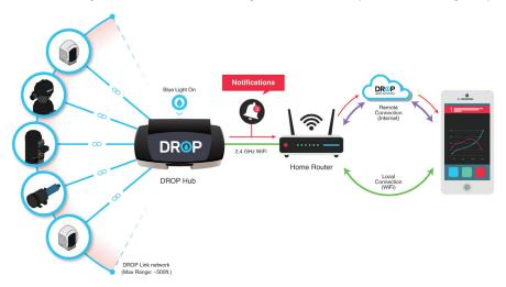
The DROP devices that are a part of your home water system are coordinated and controlled by the DROP Hub. The DROP system uses a proprietary wireless network called DROP Link that operates all the devices on a network. DROP Link is separate from and on a different frequency from your home WiFi. This gives the system resilience in that even if your WiFi or internet goes down, your DROP system will continue to operate, monitor and protect. It also keeps unnecessary traffic off your WiFi network.
