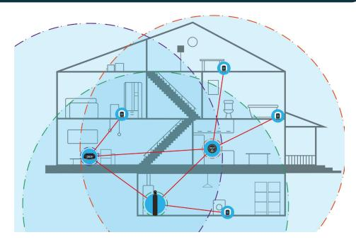
As shown above, all DROP devices that plug into 120 volt outlets expand the DROP Link mesh network. When placing the DROP Hub and Remote, keep in mind that installing them in separate areas of the home will expand the network. This is important to consider if you have leak detectors that are located in far extremes of the home. Up to 8 DROP Remotes can be added to a DROP system.
