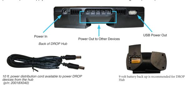
The hub also has a USB power output. This output can be used for slow charging of a tablet or phone. This is especially useful for our cabinet model where a tablet can be used for the purpose of being the user interface for the DROP system. The hub can keep the tablet charged and always ready for use.
