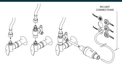
**Inlet Water Port** - Cut a short segment from the supplied 1/4" tubing ( $\sim$ 12") to install between the shutoff valve and the pressure reducer. The remaining tubing is installed between the pressure reducer and the RO System's 'FEED' port. Also, the pressure reducer needs to be installed with the arrow on the reducer pointing in the direction of flow from the water supply to the RO unit.
