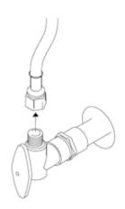
Turn off the cold water shut off valve and disconnect the supply line from the shut off valve.
